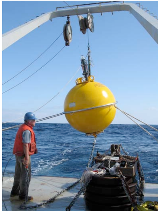
Fig. 4. Subsurface float used to support the DVLA mooring.
