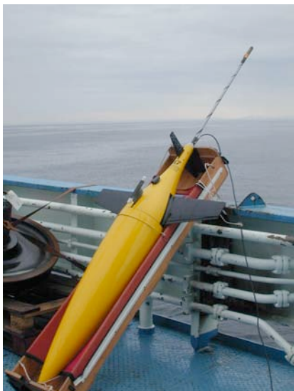
Seaglider photos. The Iridium/GPS antenna sits at the end of the long tail. Sensors are carried in the two narrow, cylindrical housings in the top aft region of the glider.
