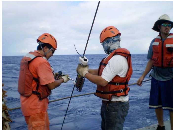
Fig 2-4. Mooring recovery procedure – Recover CTD sensors as jacketed wire reeling in.
