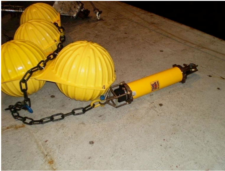
Fig 2-7. Mooring recovery procedure - Recover acoustic release.
