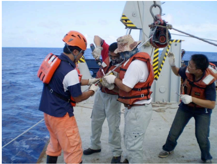
Fig 3-3. Mooring deployment procedure - Attach instrument at various depths as jacketed wire paying out.
