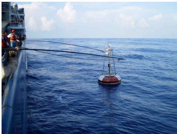
Fig 2-2. Mooring recovery procedure - Tag guide ropes to the buoy tower.
