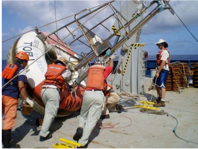
Fig 3-1. Mooring deployment procedure - Prepare buoy for deployment.
