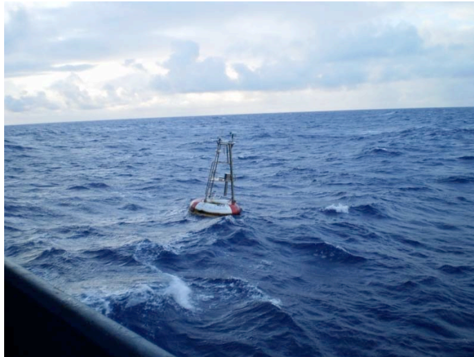
Fig 2-1. Mooring recovery procedure - Search for buoy using radar and visual.
