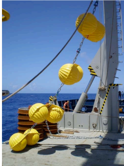
Fig 3-6. Mooring deployment procedure - Deploy glass floats.
