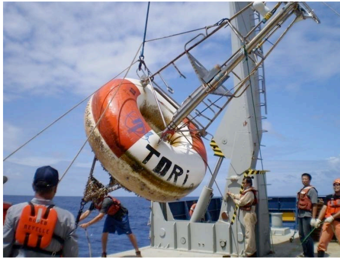
Fig 2-3. Mooring recovery procedure - Bring buoy on board with multiple safety tags.
